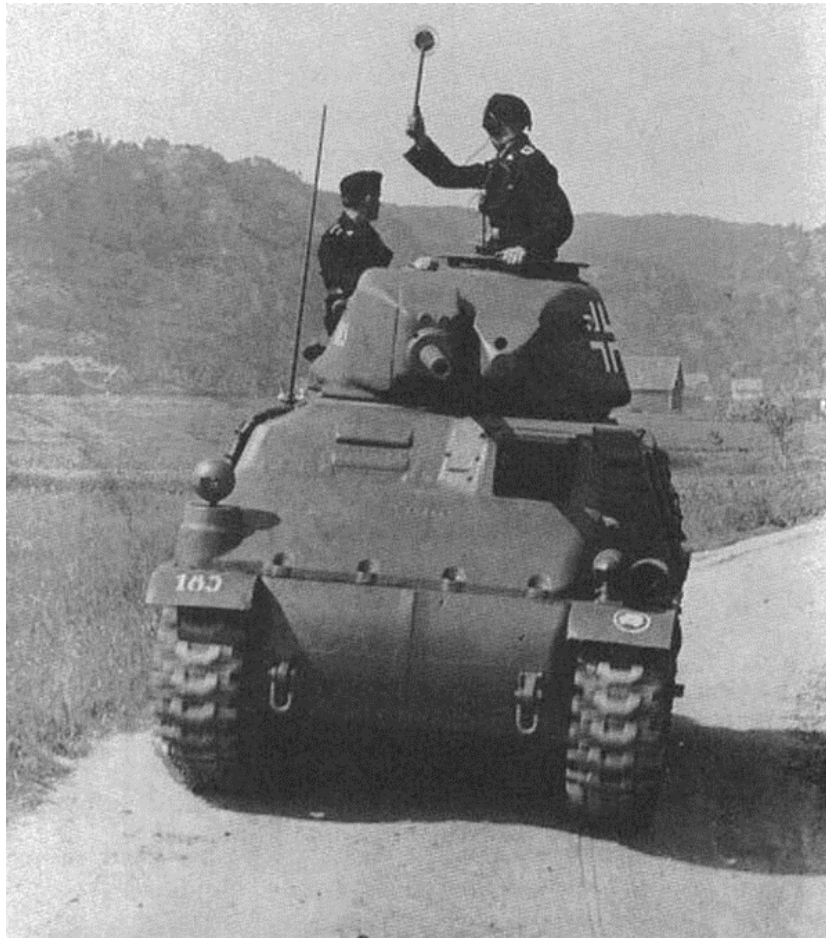
Panzerkampfwagen Somua S-35 with Pz II commander cupola. This tank, captured by the Germans after the Fall of France, was used for training and rear-echelon security duties
